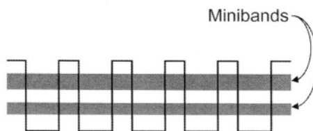
FIGURE 6.13. Schematic diagram of a superlattice structure (e.g., GaAs/AlGaAs); the gray bands correspond to miniband energy ranges.
