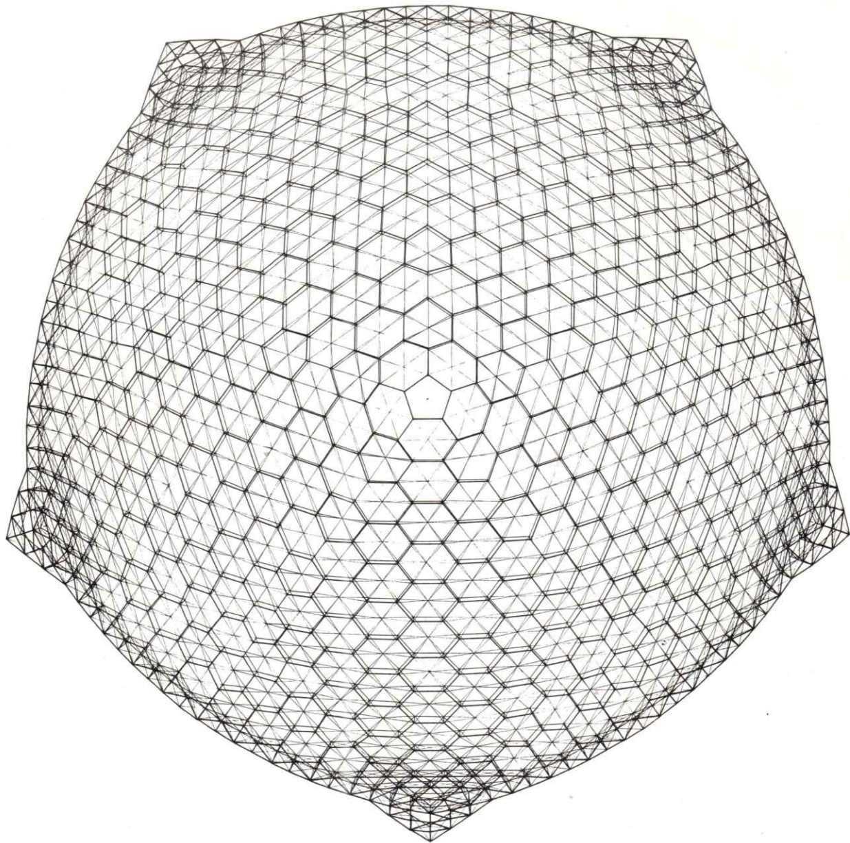
Fig. No. 70 Plan 24 V Triacon hex-pent. Double grid receives stabilization through sub guy assemblies, see Fig. 52. Pents located at zenith and in the middle of each support leg.
