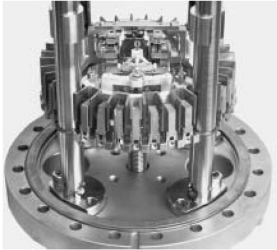
Fig. 1.9 Scanning tunneling microscope. The instrument is mounted on a flange for operation in ultra-high vacuum ( photo Omicron nanoTechnology)
