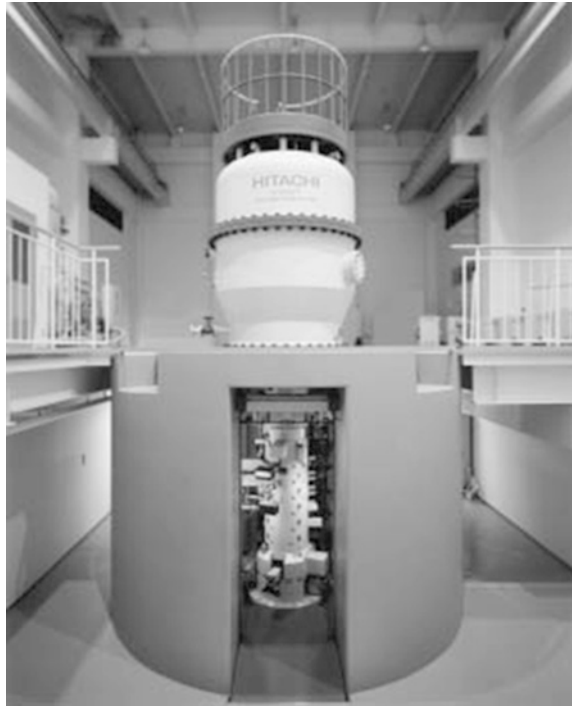
Fig. 1.8 Modern electron microscope with an accelerating voltage of one million volts ( photo A. Tonomura)
