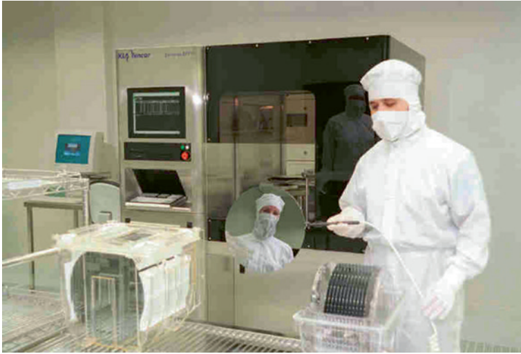
Fig. 6.9 Processing of the silicon wafers with 30 cm diameter. ( photo Wacker Chemie AG)
