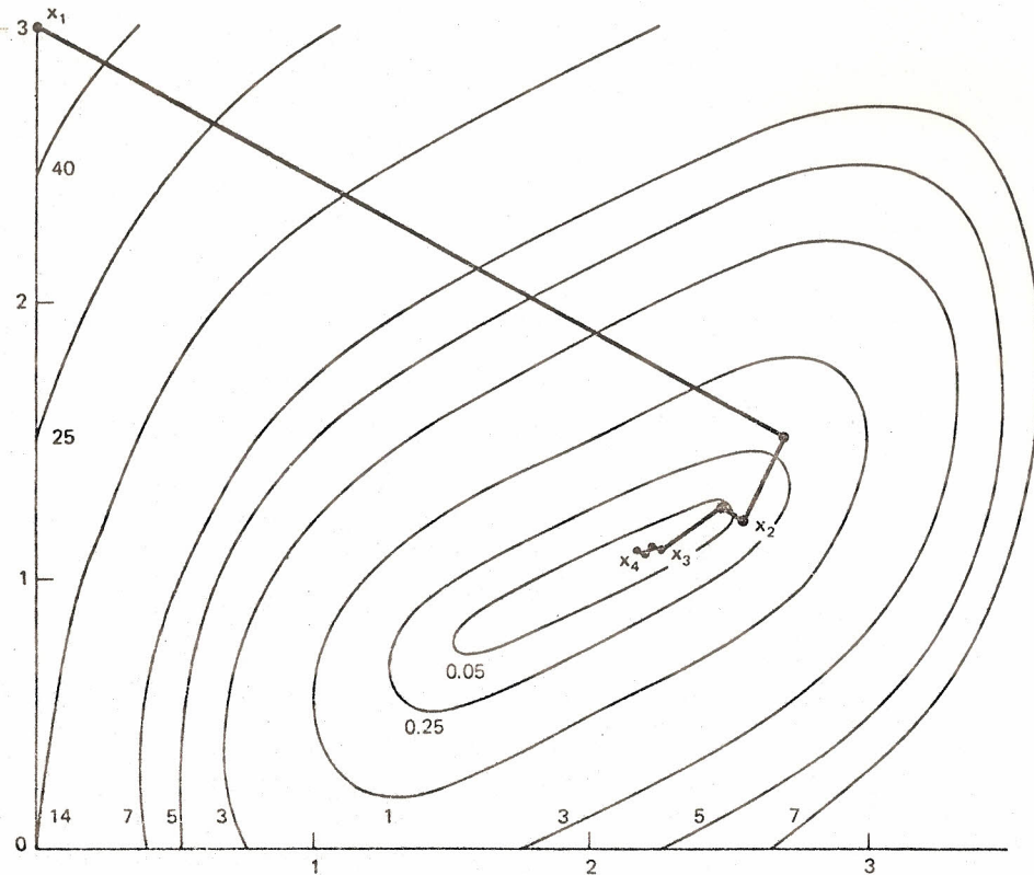
Figure 8.18 Illustration of the method of Fletcher and Reeves.
